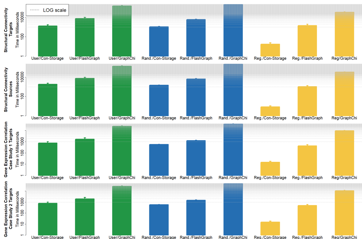
Figure 10: Comparison of query speed with state-of-the-art tools. Bars show the mean query-time with standard error of 10 user-defined VOI queries (green), 100 random VOI queries (blue) and 10 region VOI queries (yellow), for the Connectivity Storage, FlashGraph and GraphChi. The bars are log scaled, indicated by equidistant grey dotted lines (distance between two lines represent 1 second).
