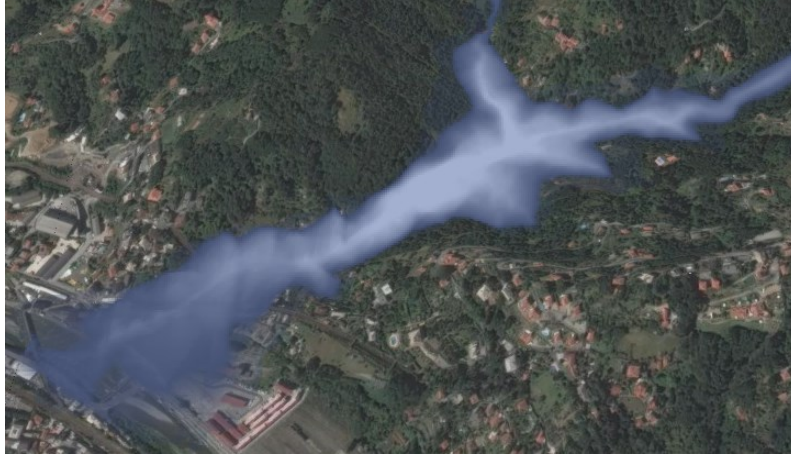
Figure 6.7.: Streaming remote visualization of an interactive flooding simulation running at interactive rates. The simulation results are composited with the terrain geometry on the browser-based client described by Bormann et al. [BGM19].
