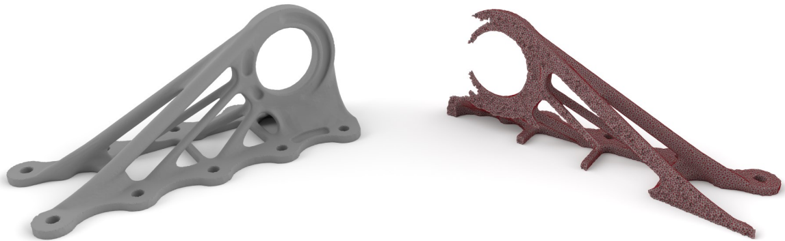
Figure 4.1.: Left: outer surface of the high-resolution mesh with 1.7 million tetrahedra used in the evaluation of our method. Right: cut through a lower-resolution model to show its inner structure. The models are based on the Airbus FCRC bracket, a titanium 3D-printed part developed using simulation and topological optimization (see, e.g., [Kra17]).
