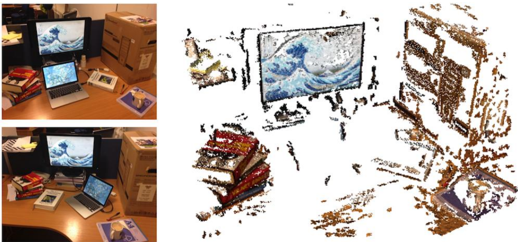
Figure 3.2: Result of directly running Structure-from-motion on images of a dynamic scene (using [115]). Note, how the algorithm misses moving objects due to its static scene assumption.
