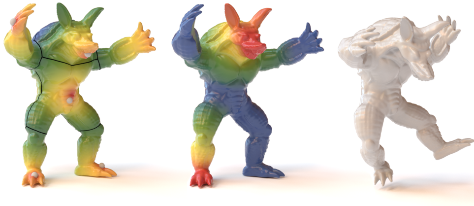
Figure 3.12: Voronoi diagram of handles (left), two weight functions (center), posed model (right).
