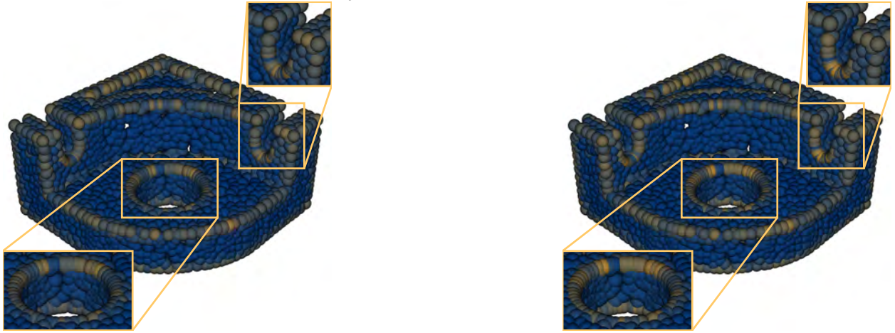
(b) Maximum principal curvature of the bearing model with weights \omega_{ij}^{\text{tau}} (6.17) on the left and \omega_{ij}^{\text{RBF}} (6.18) on the right. Note how the weights \omega_{ij}^{\text{RBF}} recover more points of low curvature in the area highlighted in the lower left and assign higher curvature to the tightly curved area highlighted in the upper right.
