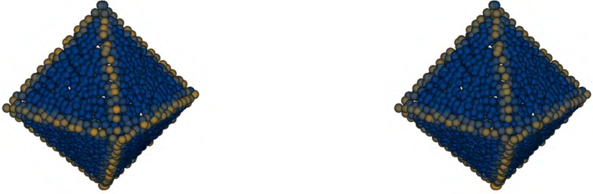
(a) Maximum principal curvature on a noisy octahedron with weights \omega_{ij}^{\text{tau}} (6.17) on the left and \omega_{ij}^{\text{RBF}} (6.18) on the right. Note how despite the noise, weights \omega_{ij}^{\text{RBF}} still capture the edges of the octahedron uniformly and the corners more precisely than weights \omega_{ij}^{\text{tau}} .
