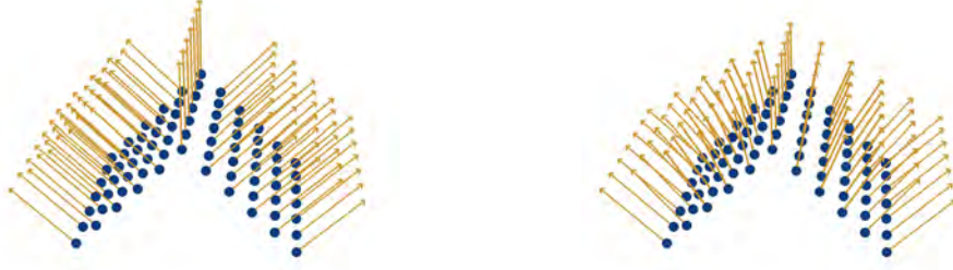
Figure 8.3: Example for a geometry, where binary values of the eigenvalues \lambda_{i,\ell} are necessary to retain the edge. See the right image, where the normal field is smoothed away despite the perfect input shown in the left image.
