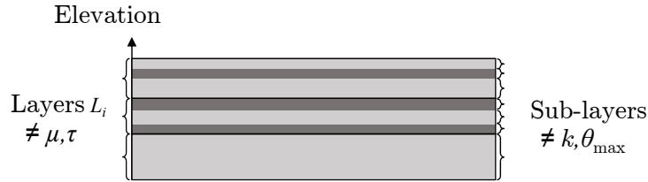
Figure 4.3: The initial stratigraphy: rock layers L_i have different mechanical properties, whereas sub-layers differ by erosion parameters only.
