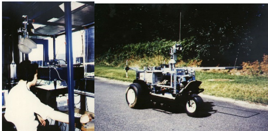
Figure 6: Head-linked stereo display providing a sensation of driving a televehicle as if on board the vehicle (left), and the mobile telexistence vehicle (right).
