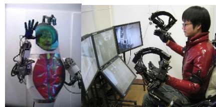
Figure 11: Mutual telexistence surrogate robot TELESAR II (left), and an operator at the telexistence cockpit (right).
