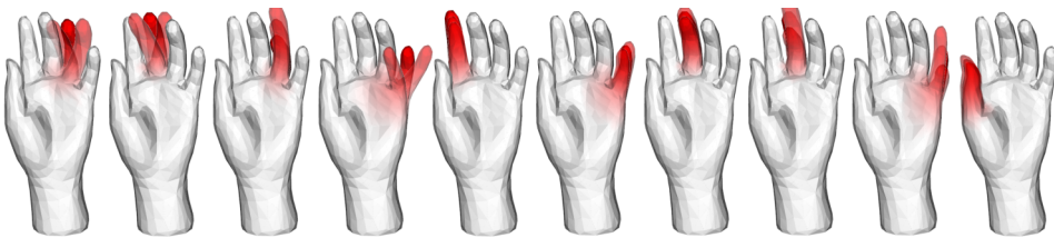
Figure 5.11: Sparsity constrained vibration modes of a hand mesh.
