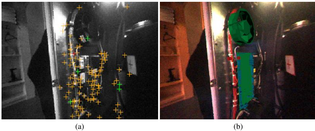
Figure 5.9.: Tracking an industrial object with the sensor fusion approach. In (a) the tracked features are colored green, feature of the model not selected for the tracking step are orange. In (b) the same frame is visualized together with an augmentation.
