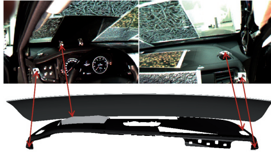
Figure 6.3.: Images from the video sequence during preparation. To increase the accuracy of the preparative SfM-based reconstruction and to reduce jittering of the camera pose tracking during HUD calibration, we attached highly textured patterns on the outer side of the windshield. At points that are accurately identifiable in the CAD model, additional marker points were placed (marked with arrows). These were used for scaled Euclidean transformation of the feature map to the vehicle coordinate system.
