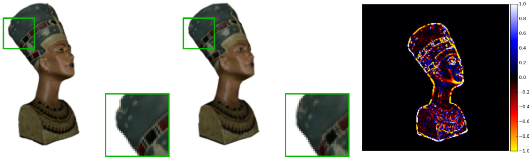
Fig. 4.10.: Visual comparison of two 200 \times 200 pixel views. Left: Full-resolution mesh (440,297 triangles, vertex colors). Center: Simplified 3D thumbnail (786 triangles, 256 \times 256 pixel texture). Right image: squared difference, multiplied by factor 8 for visualization. (Image: [LBFK15])
