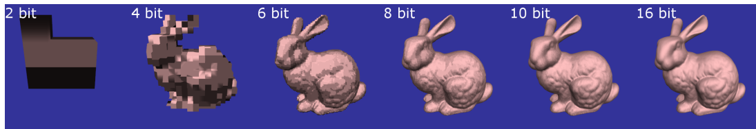
Fig. 5.4.: Streaming levels of detail, using PBG. For each level, precision of the vertex positions is indicated. Normals in spherical coordinates use half of this precision. (Image: [LJB*13])
