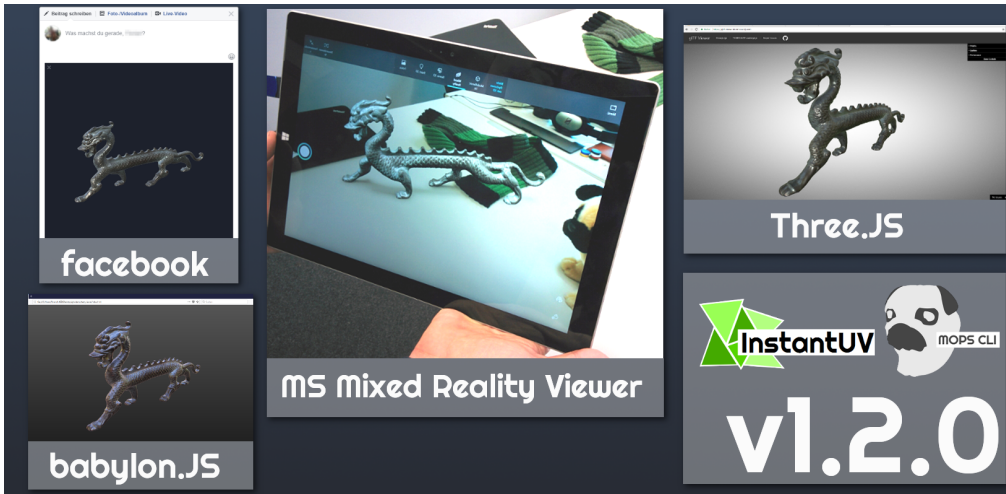
Fig. 6.2.: Optimized 3D model exported in binary glTF format and visualized using a variety of renderers. Optimization has been performed fully-automatically, using the InstantUV software.
