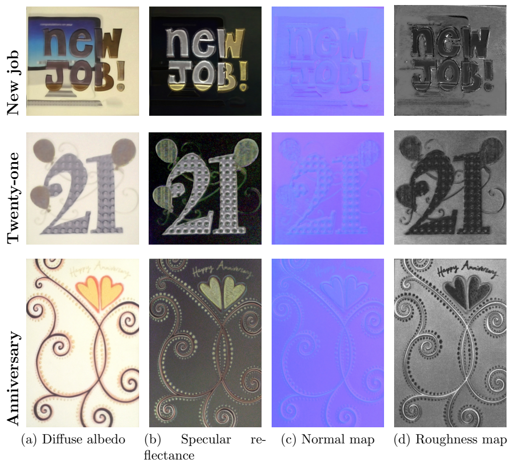
Figure 3.6: Free-form acquisition - maps: Reflectance maps recovered from our free-form acquisition setup for three spatially-varying rough specular greeting cards.
