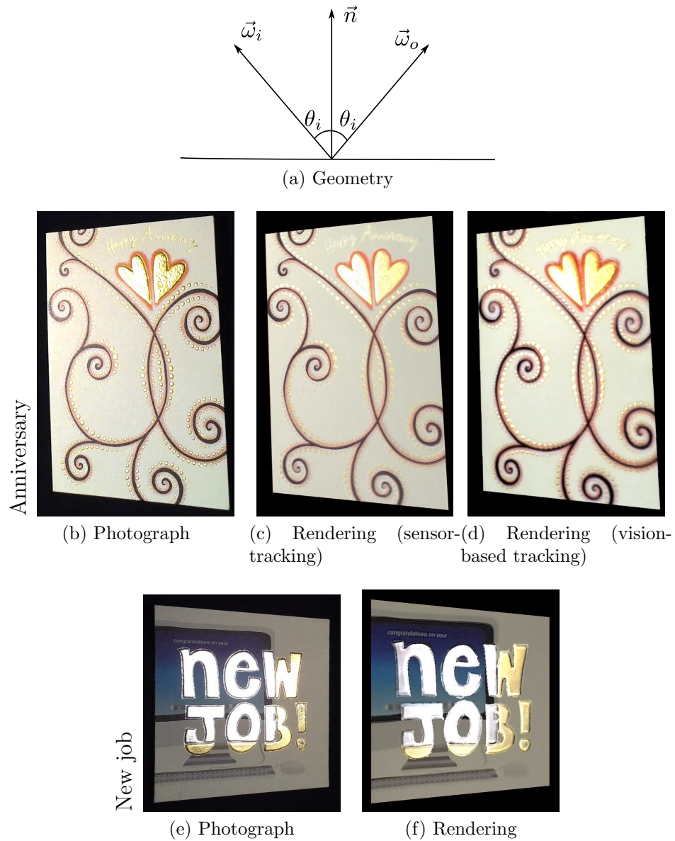
Figure 3.11: Mobile Surface Reflectometry - validation: Comparison of renderings with normal maps obtained from sensor-based tracking (c) and 3D tracking (d), to a photograph (b). Here, we also demonstrate good photo-rendering matching for novel view renderings ((b)-(f)) in the mirror direction (a).
