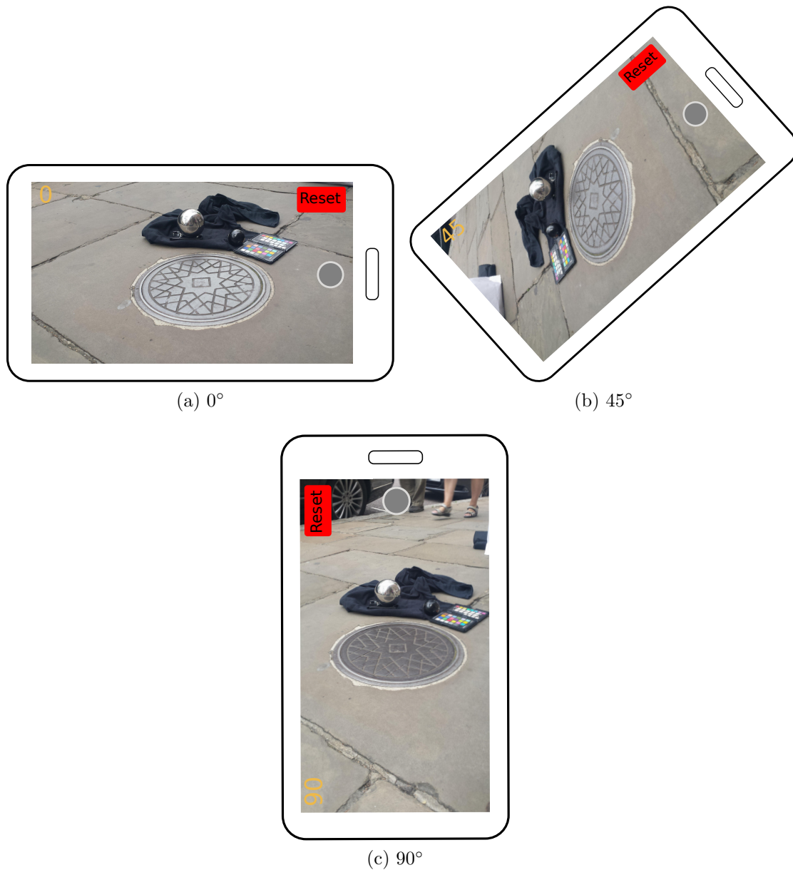
Figure 6.15: Mobile polarimetric acquisition: The user rotates the device at 0^\circ (a), 45^\circ (b) and 90^\circ (c) in order to sample the TRS. Notice how the intensity of the reflection on the “drain cover” changes with the orientation of the device.
