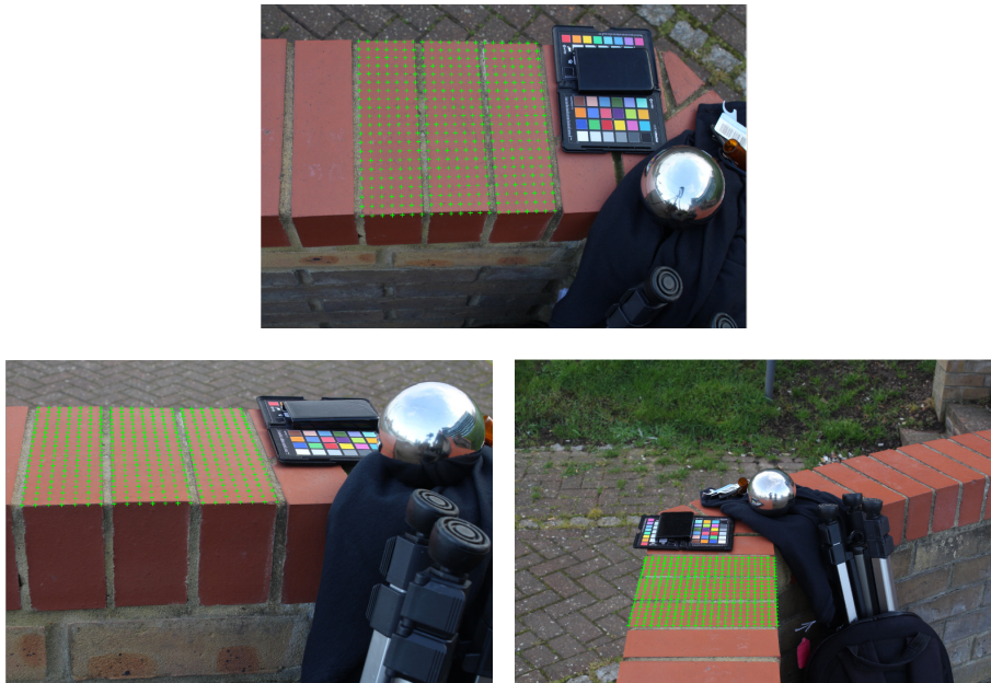
Figure 6.3: Semi-automatic registration tool: The user selects four matching corners on each frame and our tool automatically generates a regular grid of matched points ready to pass as input to VisualSfM.
