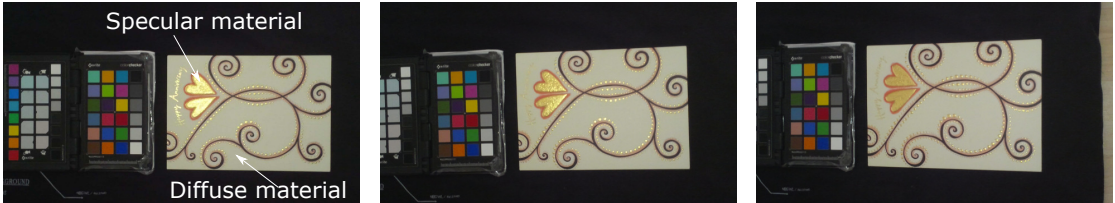
Figure 2.2: Diffuse vs Specular reflection: Notice how the diffuse material looks identical as the camera moves while the specular material changes rapidly as the camera is tilted to the right.
