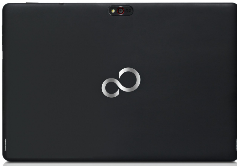
Figure 3.1: Acquisition setup: 10” Fujitsu Stylistic M532 Android tablet with an 8 MP back-facing camera with co-located LED flash.
