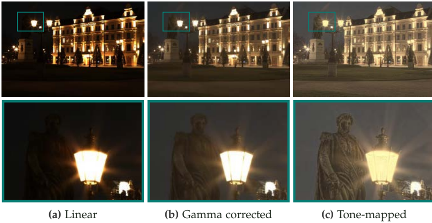
Figure 1.3: Difference between scene-referred linear values (a), gamma corrected display-referred pixels with \gamma = 2.2 (b), and a locally tone-mapped image (c), using the method from Paper C. The tone-mapping can compress the dynamic range considerably, while retaining local contrast by means of local processing.
