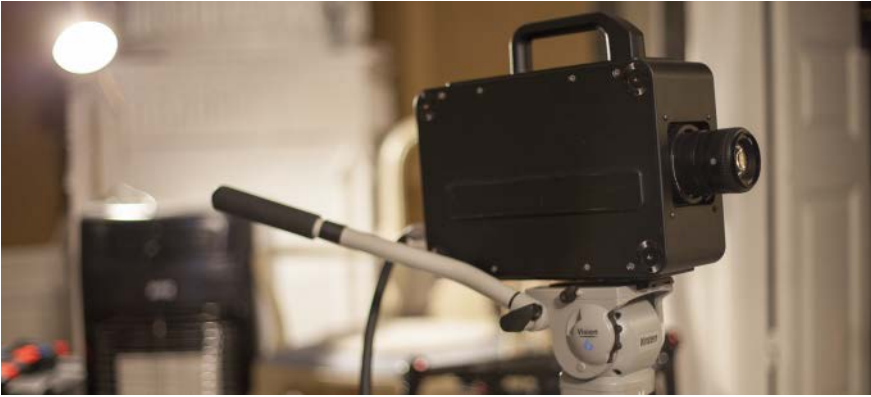
Figure 2.2: Multi-sensor HDR video camera developed in collaboration between Linköping University and SpheronVR [136], capable of capturing a simultaneous dynamic range of up to 24 stops.
