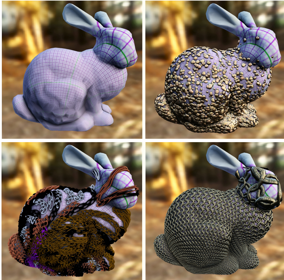
Figure 6.1: The presented warping process can be used on arbitrary U/V parametrization. However, it has to be taken care of distortions within the parametrization in order to get a consistent mapping.
