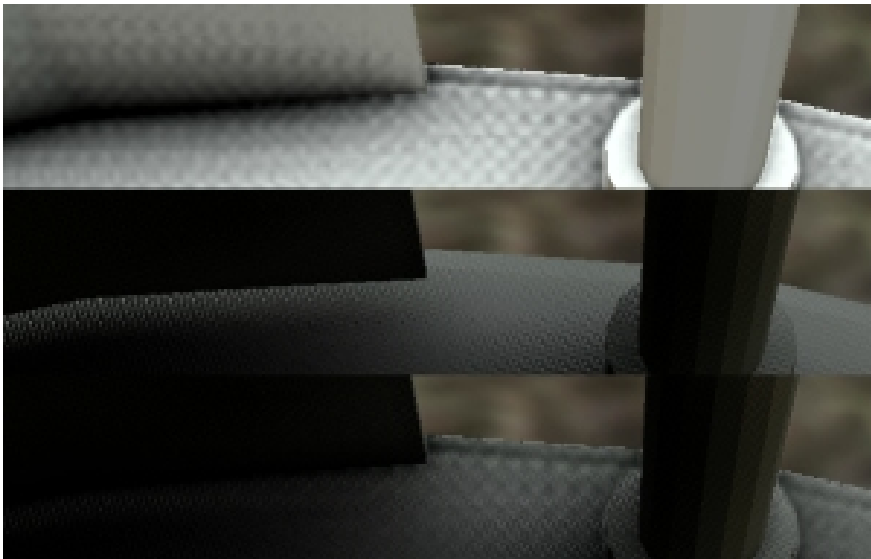
Figure 5.26: Light bleeding reduction introduced by the local part. Top: local output. Middle: global part output. Bottom: the final combination. The pattern-like artifacts visible in this images are introduced by the sampling method. Both shadow and ambience data is sampled by a dithering pattern which is visible within the magnified image region.
