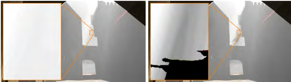
Figure 7.6: A scene rendered using prefiltered single scattering with six moments. As a dragon enters, crepuscular rays are not only darkened below but also above it. Magnified insets stretch contrasts by a factor of four.
