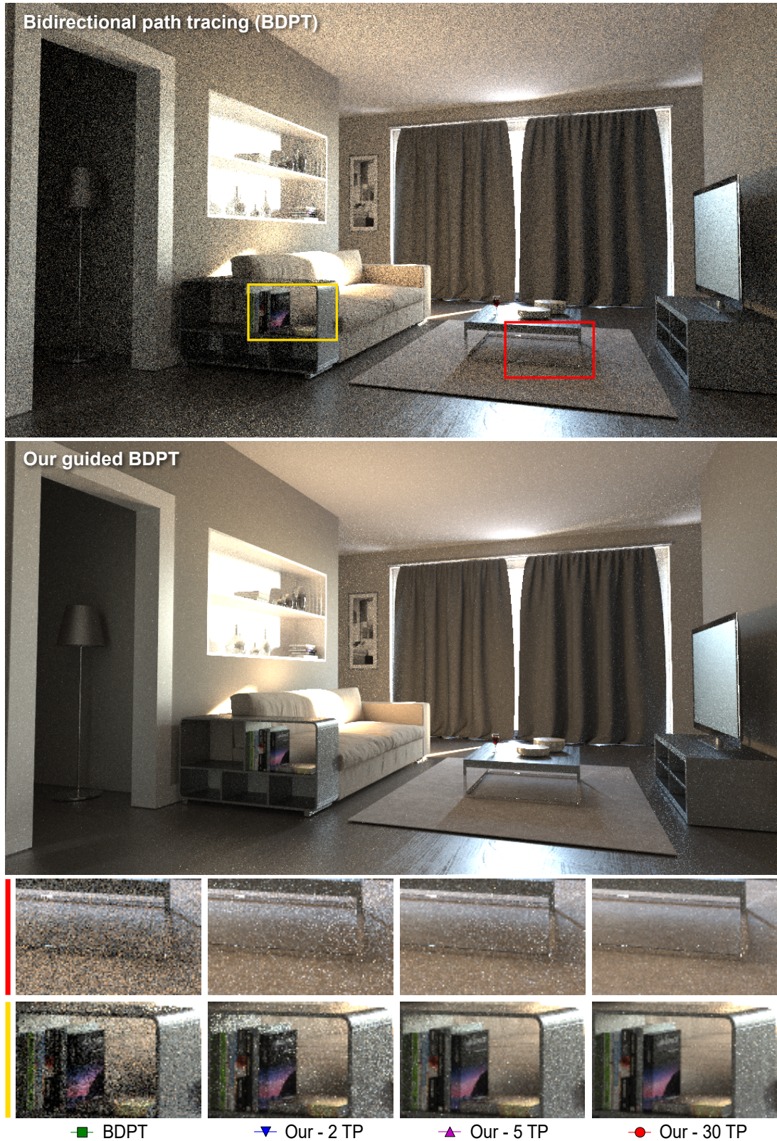
Figure 3.1: We render a scene featuring difficult visibility with bidirectional path tracing (BDPT) guided by our parametric distributions learned on-line in a number of training passes (TP). The insets show equal-time (1h) comparisons of images obtained with different numbers of training passes. The results reveal that the time spent on additional training passes is quickly amortized by the superior performance of the subsequent guided rendering. Convergence plot corresponding to these four methods is shown in Fig. 3.2.
