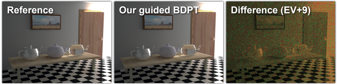
Figure 3.11: Our method converges to the reference image computed by plain BDPT (left). We rendered the scene for approximately two days with our guided BDPT that used 30 TP (middle). The reference image was rendered by BDPT for approximately 10 days. The uniform distribution of positive (green) and negative (red) differences (right) suggests that any residual error is only due to variance. Brightness of the difference image was multiplied by 2^9 .
