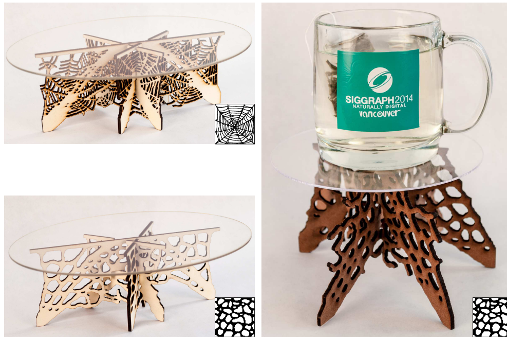
Figure 4.35 – Three tables produced with our system, using three planks and structures optimized independently. The two tables on the left use the same external conditions but different patterns. The right table weights 76 g and is supporting a filled cup of 762 g (10× heavier).
