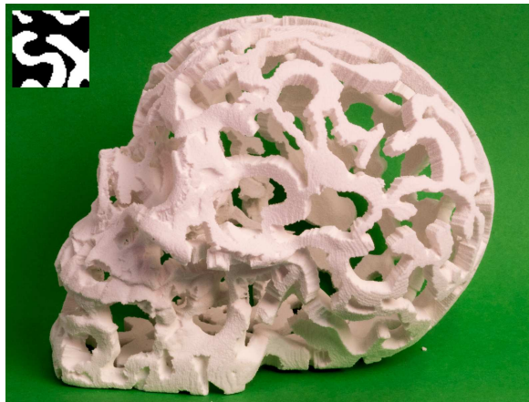
Figure 4.14 – Result printed on a ZCorp 450. On this type of machines the printed objects are very fragile and have to be extracted from the powder bed before dipping into cyanoacrylate. Our thin patterns nevertheless print successfully.
