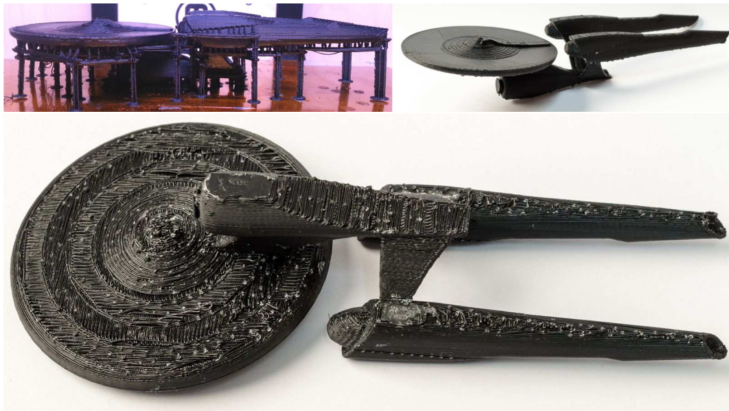
Figure 3.10 – Top: Printout of the Enterprise model. Bottom: Under-side after cleanup. We broke the engine connectors during cleanup and had to glue them back (only case where glue was involved). Print time: 3 h 14 min, 9.89 m of filament.
