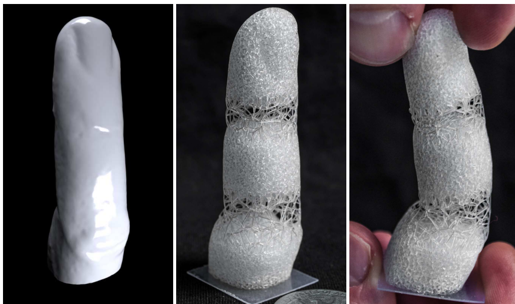
Figure 5.14 – Finger with articulations. Right: deformed object. Note that the inferior articulation is made wider and thus bends further. Model: Olivier hand (AIM@SHAPE Project).
