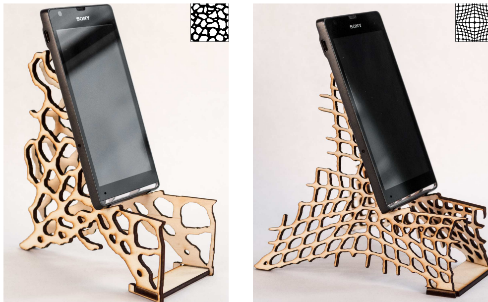
Figure 4.34 – Phone stands fabricated from optimized structures using two different exemplar patterns.
