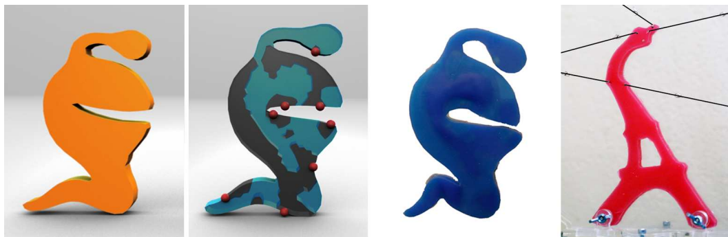
Figure 2.10 – Synthesis of deformable characters [Skouras et al. 2013]. A material distribution mixing two different materials is optimized, so the fabricated shape can deform according to a prescribed scenario. The characters are then animated using a small number of actuators.
