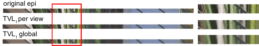
Figure 4.1: Visualization of the horizontal epi view for the red scanline in Figure 4.2 (a). From top to bottom: the epi from the original light field; the epi after applying TVL 1 filter to each view separately; the same epi after applying a 4D TVL 1 filter to the whole light field volume using our approach. We can observe (by zooming in the digital version), areas with very similar colors are flattened, while sharp discontinuities are preserved, effectively removing noise and promoting angular coherence.
