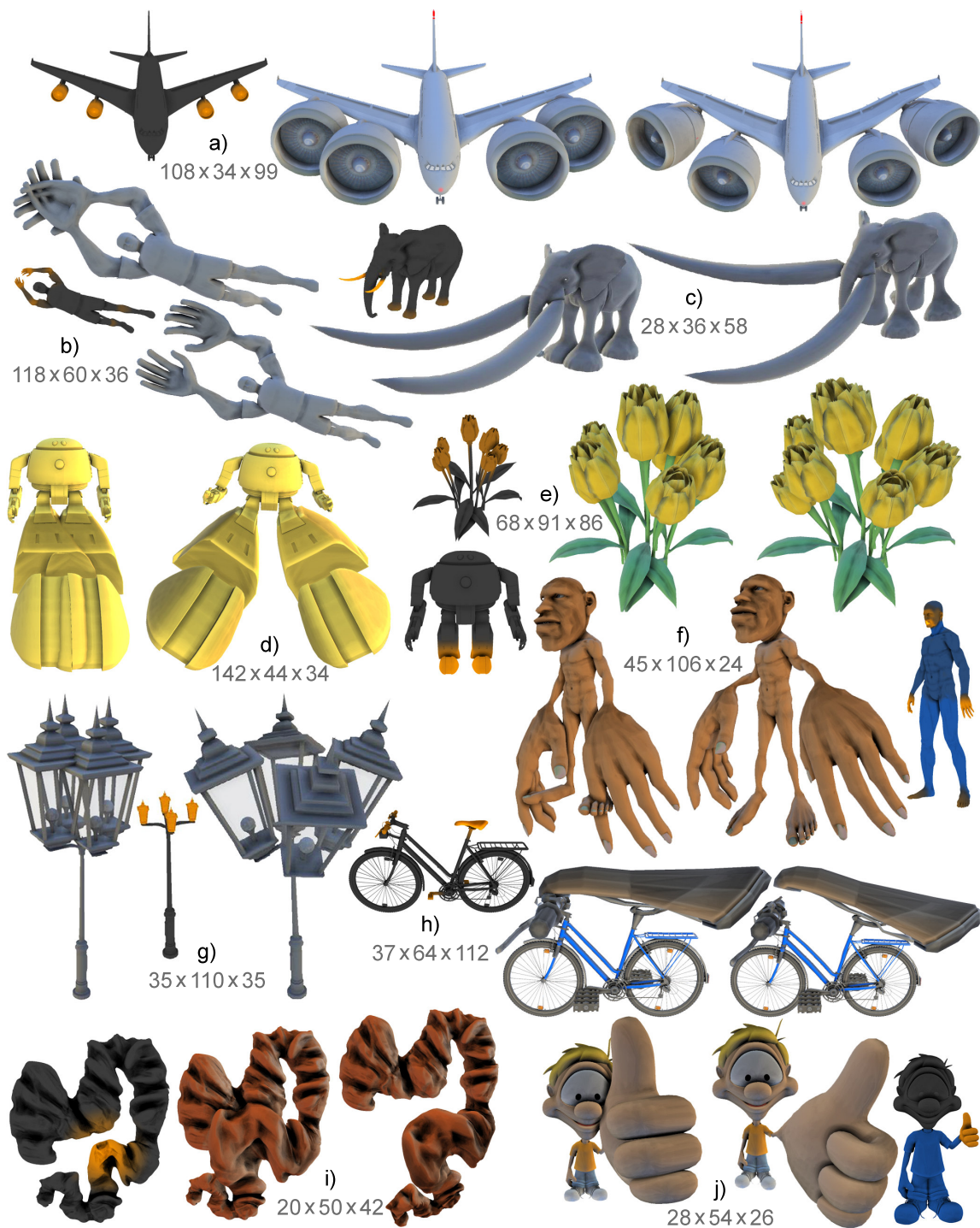
Figure 3.7: Results of classic deformation ( Left ) compared to our collision-aware approach ( Right ). For every example the resolution of the voxelization is listed and a false-color coded importance field is shown. a) : Noise sources of an airplane. b) : Injury probability of a goal keeper c) : Black market price of body parts of an elephant. d) : Force field on a robot. e) : Pollen concentration of flowers. f) : Homunculus. g) : Heat field on a street lamp. h) : Diluent concentration of bike parts in contact with human body. i) : Focus+context visualization of a colon model (cf. [Wang, Lee and Tai, 2008]). j) : Comic character deformation.
