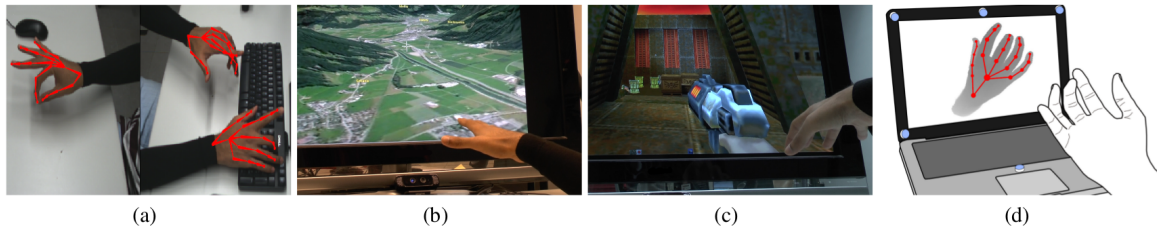
Figure 7.1 (a) FullHand can track one or both hands with all fingers. (b, c) FullHand enables free-hand interactions for many applications such as virtual globes and first-person shooters. (d) We envision miniature multi-camera setups for hand tracking in the future. The blue cylinders represent cameras.
