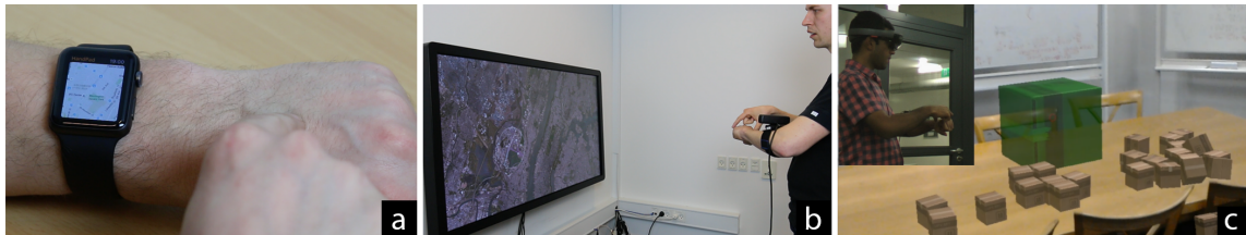
Figure 9.7 Some interactive applications enabled by WatchSense . (a) Single-touch input allows for panning a map on a smartwatch. (b) Multitouch allows for zooming/resizing a lens on a large display. (c) Compound touch and mid-air interactions allow for more expressive input for emerging mixed reality devices. Here we show a user interacting with virtual boxes through a HoloLens.
