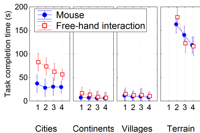
Figure 7.10 Development of task performance for mouse vs. free-hand interactions in four navigation tasks with the Virtual Globe. Vertical bars denote 95% confidence intervals.
