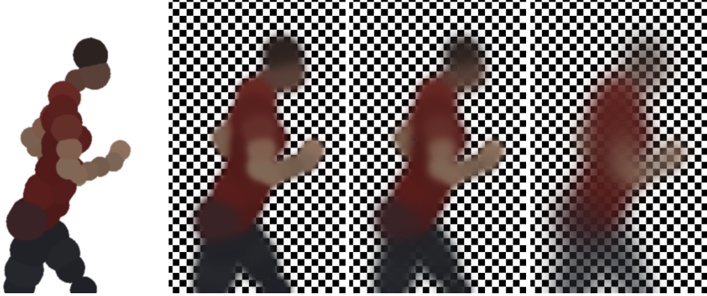
Figure 4.2: From left to right: A solid sphere actor model, our representation by a translucent medium with Gaussian density visualized on a checkerboard background for increasing smoothness levels ( m=\{0.0001, 0.01, 0.5\} ). Note the proper occlusion, e.g. of the left arm and the torso.
