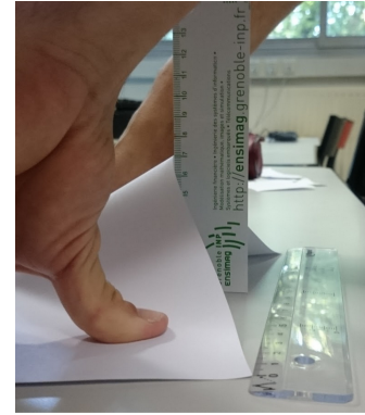
FIGURE 3.12: Experimental evaluation shows that our cone deformation model produces results that correspond to real paper.
