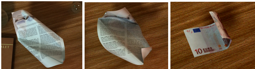
FIGURE 4.22: Different paper materials being crumpled can be synthesized in recording different databases: (Left) printer paper, (Middle) tracing paper, (Right) a bank note.
