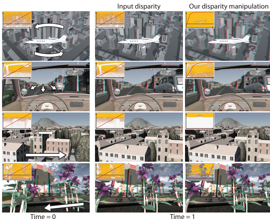
Figure 7.5. Results of our parallax-aware disparity manipulation applied to four video sequences used in our user study (Sec. 7.3.1). Two frames from the input sequences ( 1st and 2nd columns ) compared to our outputs at Time = 1 ( 3rd column ). The mapping curves along with the output disparity maps are shown in the insets. The blue color marks crossed disparity, yellow uncrossed disparity and white zero disparity. The arrows show the local motion direction.
