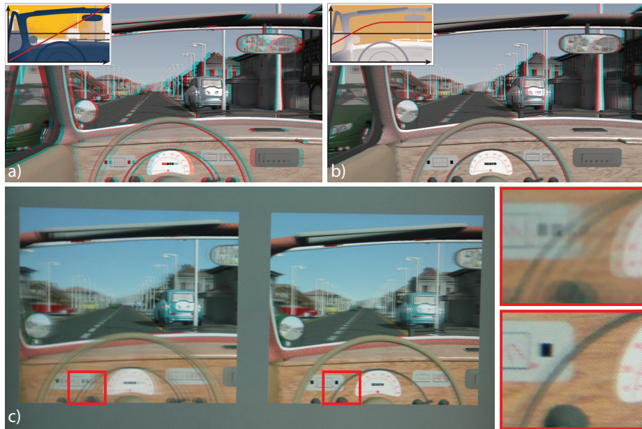
Figure 7.6. Example of disparity compression for autostereoscopic displays. a) The original linear compression with the corresponding disparity map and mapping curve shown in the inset. b) Our manipulation applied on the top of (a) to compress stronger regions that benefit from motion parallax. c) A photo of our display. Aliasing artifacts are strongly present in the content with only linear mapping (insets).
