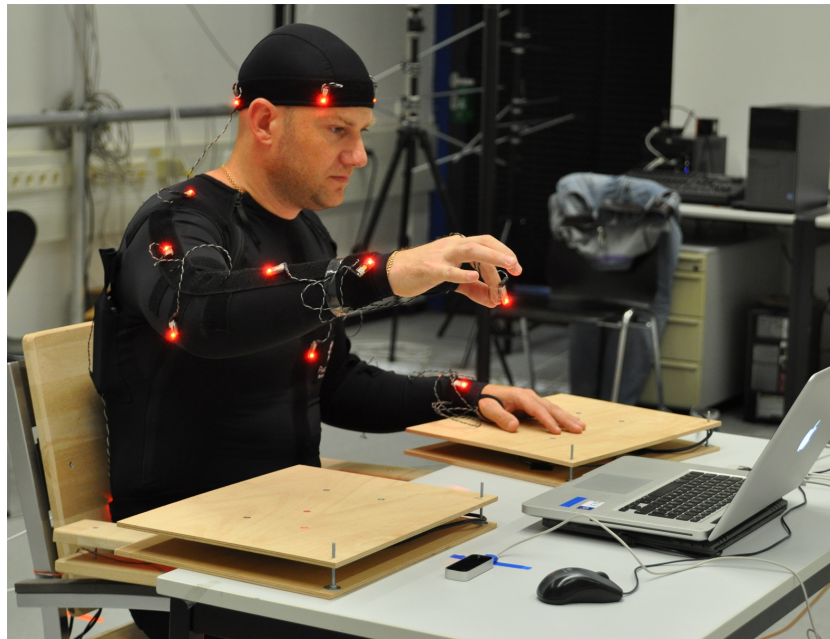
Fig. 2.4: Optical motion capture and external force recording during mid-air gestural interaction.
