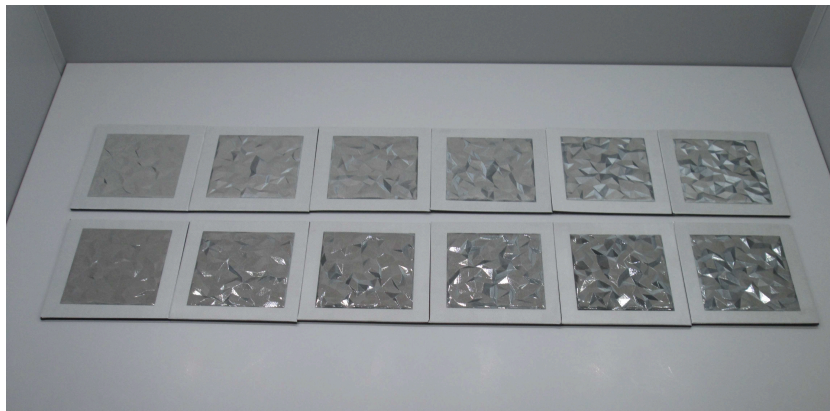
Figure 6.20.: Two sets of 2.5D textured reference samples with "Facet" texture type printed with minimum (first set = top row) and maximum (second set = bottom row) gloss, using 0% and 40% varnish deposition respectively. The six samples within each set have different texture levels, yet the same printed-gloss. These reference samples were used in the texture ranking and scaling psychophysical experiment.
