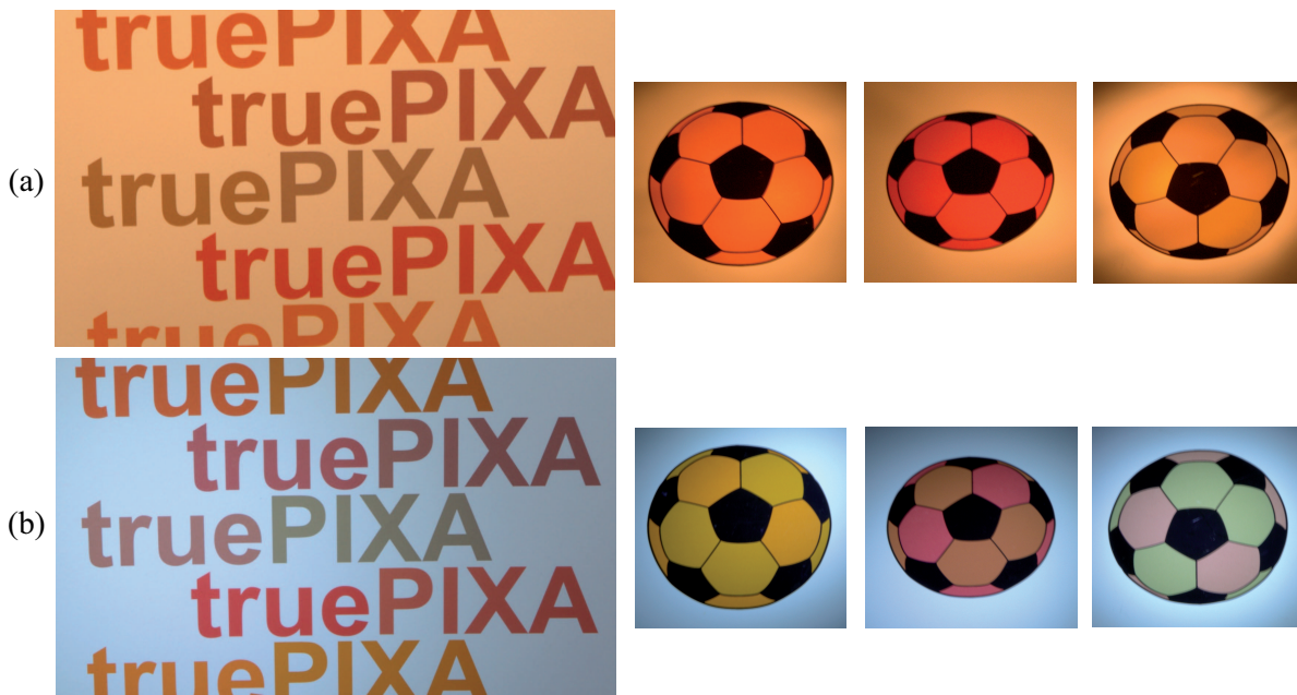
Figure 4.17.: Captured spectral prints under two light sources: (a) halogen-based and (b) LED-based flashlights. Noticeable color changes are visible in the samples of the second row. Please note that the printing and capturing process can introduce color errors. The results are more reliable in the zoomed-in electronic version of this dissertation.
