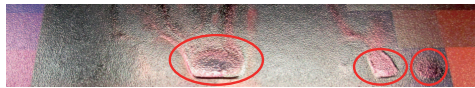
Figure 6.1.: A cutout of an image captured from a printout representing bronzing artifacts (visible in the marked ellipses) occurred due to aggregation of deposited inks.
