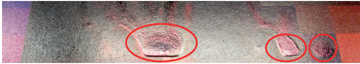
Figure 1.2.: A cutout of an image captured from a printout showing bronzing artifacts (visible in the marked ellipses), which have occurred due to aggregation of deposited inks.
