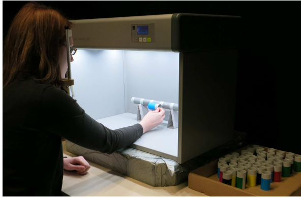
Figure 6.24.: Gloss scaling experimental setup. This figure has been taken from [SBU14].
