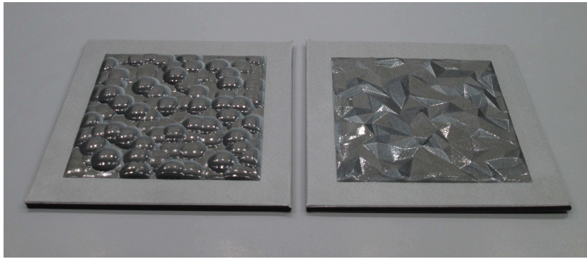
Figure 6.17.: Textured samples of Group III : (left) "Bumpy" ellipsoids and (right) macroscopic "Facet"s.
