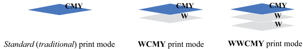
Figure 6.4.: Schematic representation of three print modes: standard , WCMY , and WWCMY . Here, (W) refers to base white layers and CMY represents the top color layer achieved via combinations of C, M, and Y inks. This figure has been taken from [BSB*14].
