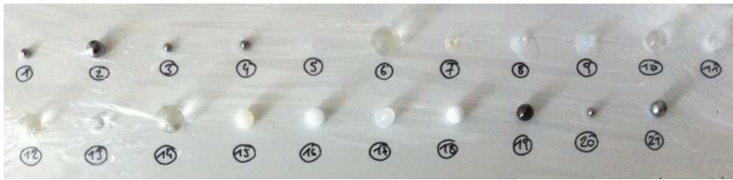
(a) Spherical fiducial makers which are made of different materials (metal, steal, glass, PA, POM, and PTFE) and have different radii (1mm to 10mm)
