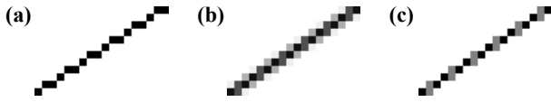
Figure 13: A line of slope 2/3 with (a) no antialiasing, (b) automatic antialiasing, and (c) manual antialiasing.
