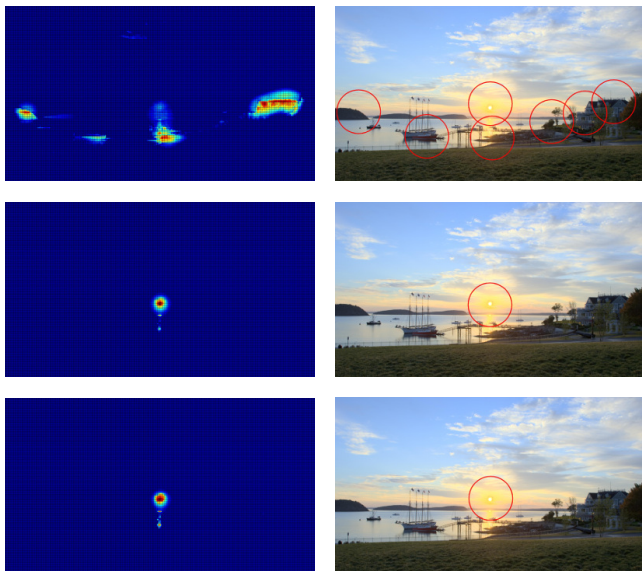
Figure 7: Comparison with other approaches. From top to bottom, saliency maps and regions of visual attention (red circles) produced by our method, the method of Itti and Koch [2000], and the method of Brémond et al. [2012]. The HDR image is from Mark Fairchild's HDR Photographic Survey, © 2006-2007 Mark D. Fairchild.
