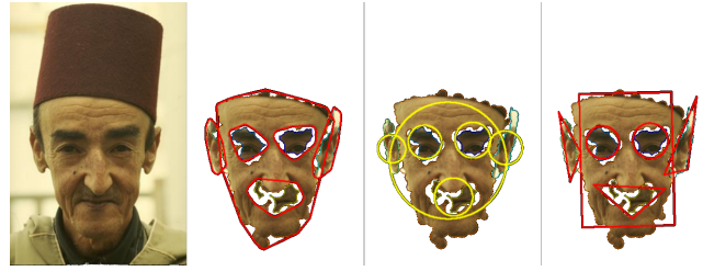
Figure 5: Fitting Shapes to Object Parts: robust convex hull, ellipses, and rectangles. (Source photograph taken from Berkeley’s publicly available database.)
