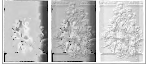
Figure 8: The chromatic image (centre) is the sum of the Cromadepth® image (left) and the shading image (right)
