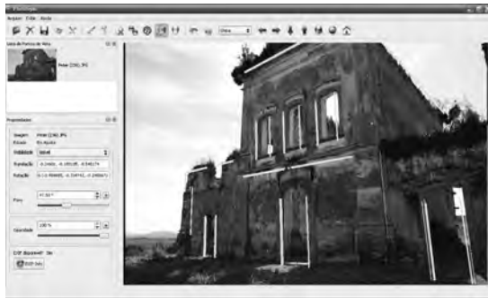
Figure 4: Model superimposed by an image with opacity of 100%. Even with maximum opacity, the guidelines are still visible and the model can be manipulated.
