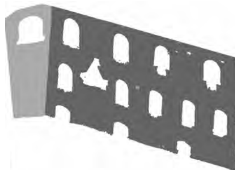
Figure 14: Segmentation results for the point cloud shown in Figure 13
