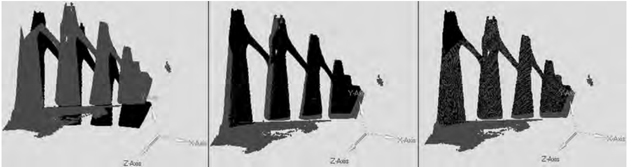
Figure 7: On the left, the reference scan (in grey) and the scan to be registered (in black) in their original positions. In the middle, the scan to be registered has been rotated by \omega_0 and is in approximate alignment with the reference scan. On the right, the results of the registration after the implementation of the ICP are presented.
