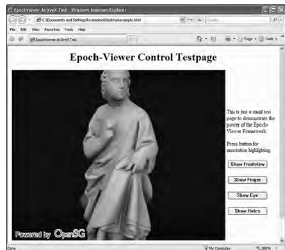
Figure 3: The Epoch-Viewer ActiveX control inserted into an HTML page using the object tag. GML functions for loading and highlighting the annotations are triggered with JavaScript.
