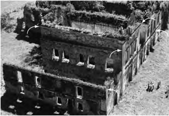
Figure 1: Example of simple vanishing point calibration. Marked lines are indicated by the white arrows.
