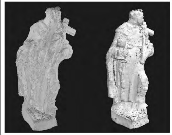
Fig. 7. Example of an image obtained directly from the reflectivity values after having merged several scans (left) and the shading image (right)
