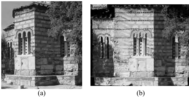
Figure 11: Orthophoto produced with the proposed method (b) using initially "oblique" image (a)
