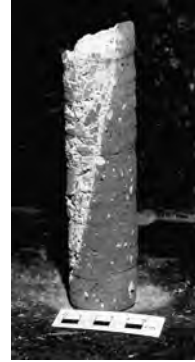
Figure 3: Colored lime-mortar containing brick dust from Hagia Sophia Thessaloniki (dated from the Byzantine period, 7 th cent. AD).
