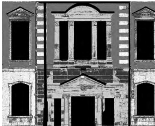
Figure 12. Building C - Classification with intensity.
