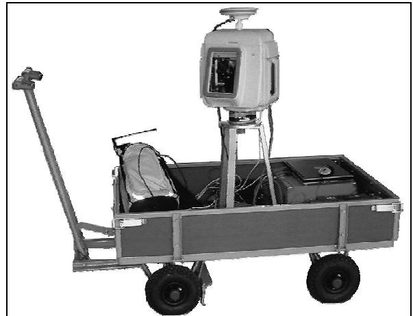
Figure 1: The Trimble® GX scanner integrated on a mobile platform
