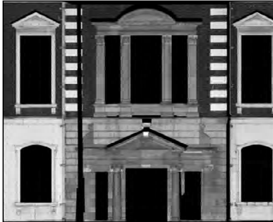
Figure 10. Backscattered Intensity represented in greyscale prior to classification.
