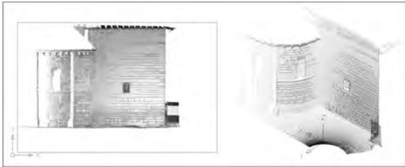
Figure 5: 2D lines over the orthoimage (left), and the same lines after projecting them over the point cloud (right)
