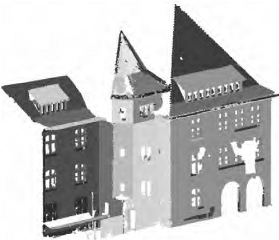
Figure 18: Adjacent façades segmented into principal planar surfaces and features
