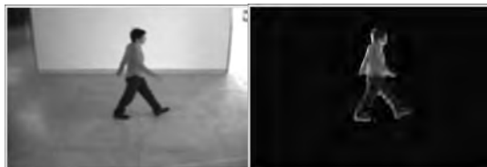
Figure 3: The results of background subtraction (the left image is an original image and the right image show the foreground image)
