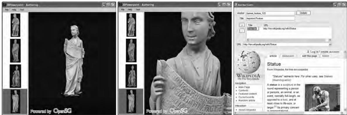
Figure 4: The showcase for authoring: The user navigates to a position of interest. Annotations are added by clicking on the model and dragging the radius of the markup sphere. In the anchor form multiple URLs can be attached by typing or dragging the address from a browser. The dialog also includes a browser for preview and web navigation. (web browser: www.wikipedia.org)
