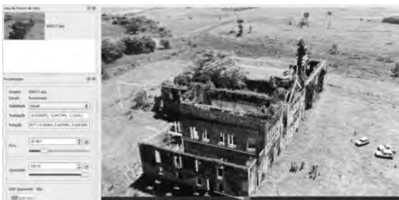
Figure 13: A match between the model and a picture of the convent. The picture is shown with 100% of the opacity. This picture was taken in the early 80's so no EXIF info is available. Vanishing point calibration was used.
