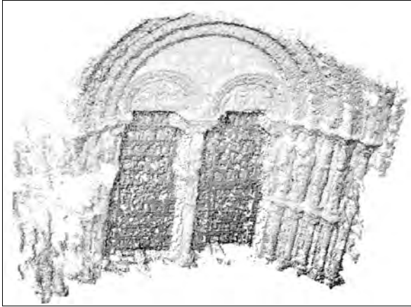
Figure 10: Unfiltered and unconstrained 3D disparity point cloud
