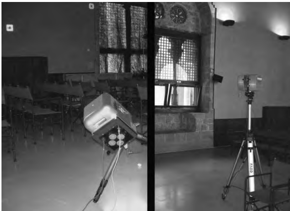
Figure 4. Laser scanning survey. Left : Mensi GS 200 and reflecting targets on the wall. Right : Faro LS880
