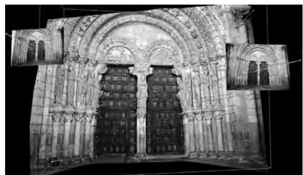
Figure 7: OpenGL “near orthophoto” 3D view. Geometrical depth noise is less noticeable in this view therefore the mesh is adequate
