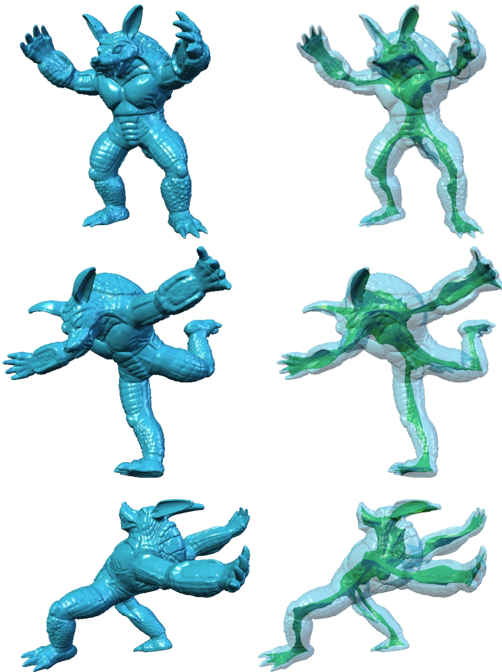
Figure 6.33: Thickness visualization of our deformations. Top-left: original Stanford Armadillo model consisting of 332K triangles. Top-right: the control mesh approximates the medial axis with its associated distance field. Middle/Bottom-left: different large-scale deformations generated using our method. Middle/Bottom-right: modified control meshes with their associated distance fields. Generating these deformations is rather fast: it takes only 0.3 seconds for deforming the coarse control mesh (5.2K triangles) and 3.8 seconds for a multiresolutional reconstruction of the deformed dense mesh.
