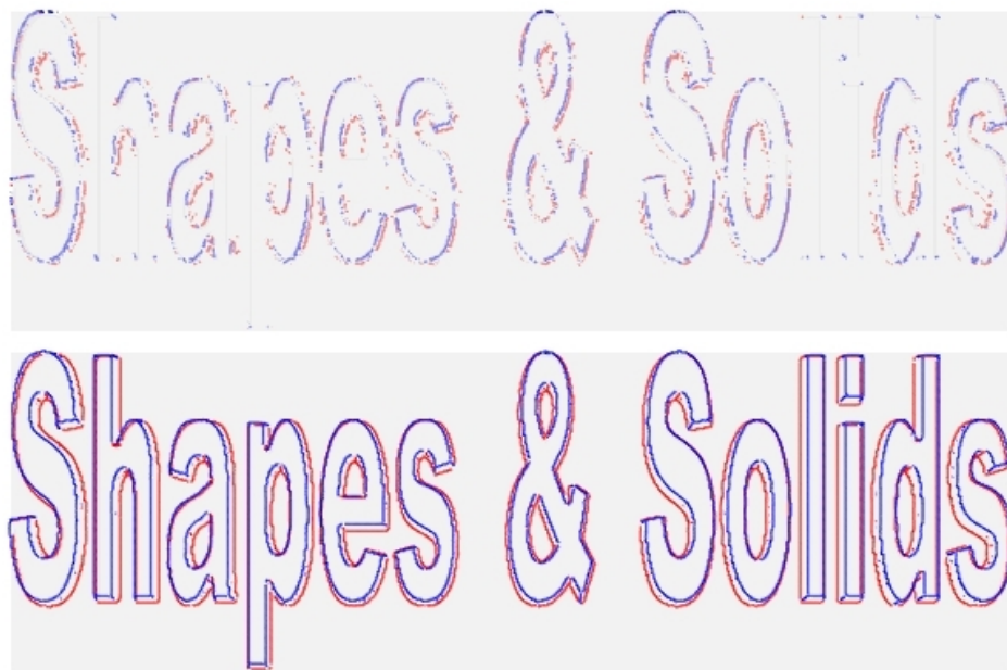
Figure 4.6: Crest lines detected on 3D text. Top: polynomial fit without preliminary estimation of mesh normals is used. Bottom: the enhanced adjacent-normal cubic approximation method is employed for estimating surface curvatures and their derivatives. In both the cases preliminary smoothing \mathbf{p} \rightarrow \mathbf{p}' was applied.
