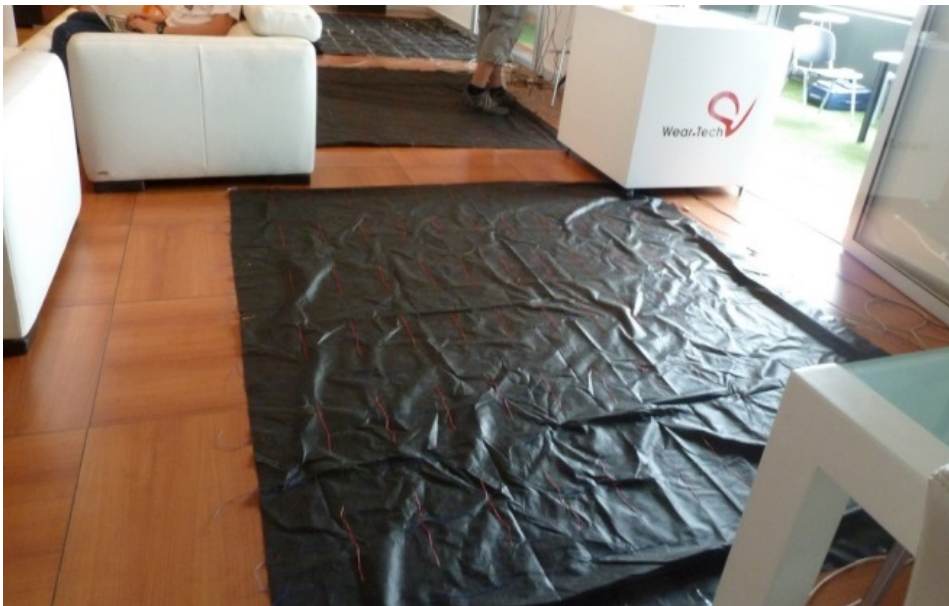
Figure 4.25.: Floor mats with integrated CapFloor system used at the EvAAL 2011 competition [BHW12]
