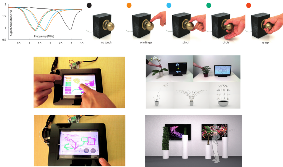
Figure 2.18.: Top : Capacitive profiles of different gestures on a door knob [SPH12]. Bottom Left : User identification using capacitive fingerprinting [HSP12]. Bottom Right : Botanicus Interacticus prototype and interaction concept [PSLS12].
