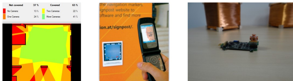
Figure 2.29.: Left : Coverage of a room by camera fields of view - AmbiTrack [BDA*13]. Middle : Fiduciary marker photographed by camera phones [MWBS09]. Right : Magnetic coils in background and receiver circuit in foreground [PL13].
