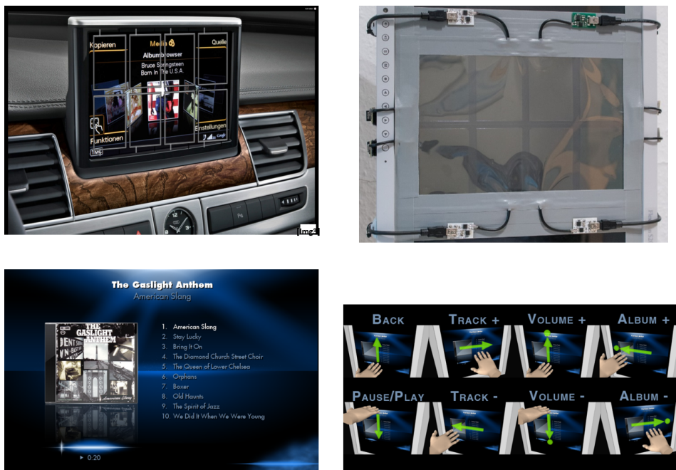
Figure 4.59.: Top left : Concept image of GestDisp in a car with outlined electrodes. Top right : GestDisp prototype installed in front of a monitor. Bottom left : Screenshot of demonstration application music player. Bottom right : Association of gestures to functions in the demonstration application.
