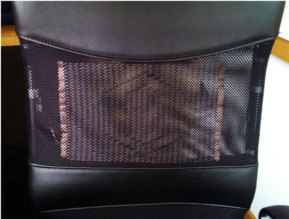
Figure 4.32.: Detail view of conductive thread electrode
