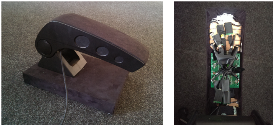
Figure 4.38.: Active Armrest prototype, left - outside view, right - detail view of electronics [BNS*14].
