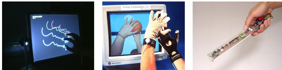
Figure 2.30.: Left : FTIR multitouch table [Han05]. Middle : DataGlove hand gesture system [ZLB*86]. Right : XWand interaction device [WS03].
