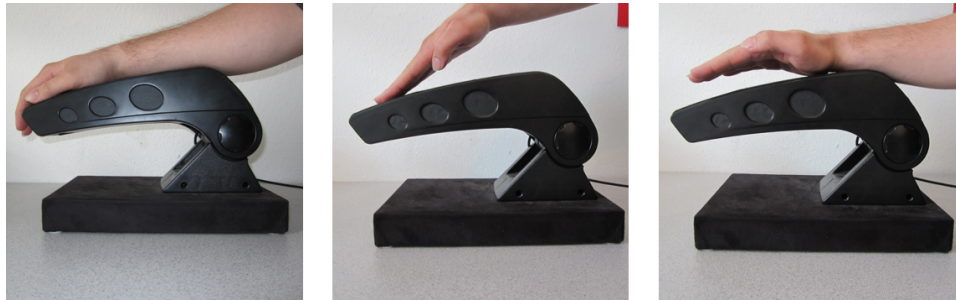
Figure 4.39.: Postures of limbs on armrest - resting position (left), arm raised position (middle), hand raised position (right) [BNS*14].
