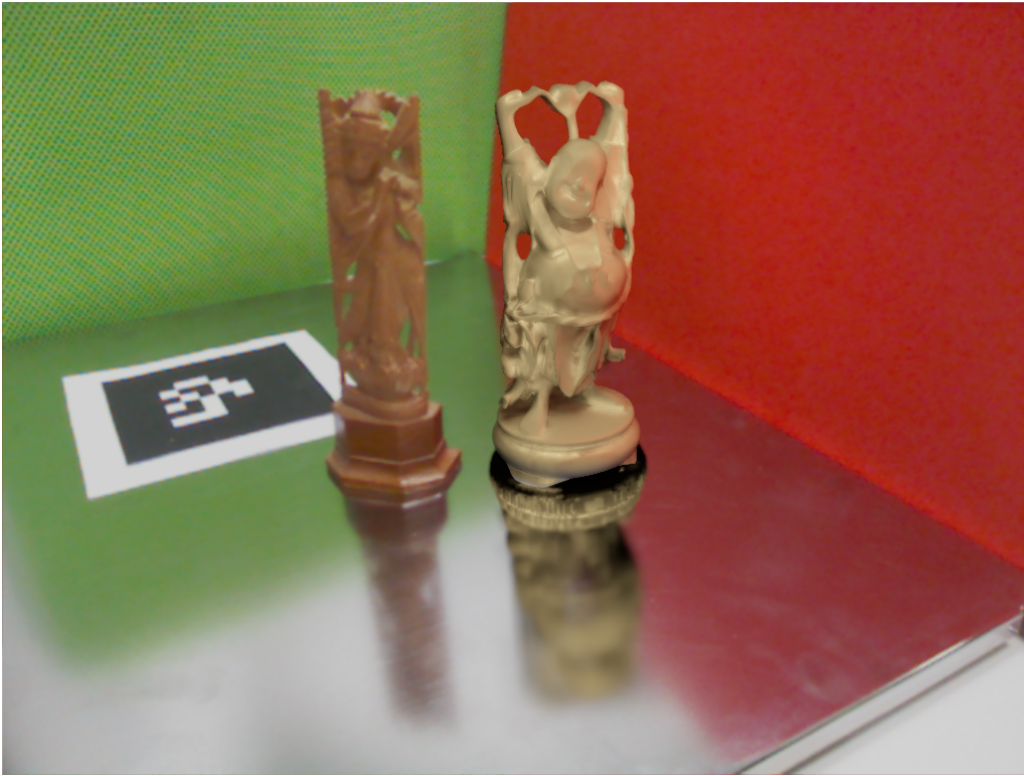
Figure 5.12: Indirect bounces, from purely diffuse to specular, are supported by DVCT. This image, rendered in 26ms, features glossy indirect reflection of the virtual Buddha in a real surface, as well as diffuse bounces from real surfaces on the Buddha.
