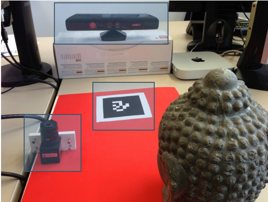
Figure 3.3: A relighting setup: The scene is recorded and partially reconstructed with a Kinect sensor. A marker is used to geometrically register the scene and a secondary UEye UI-2230-C fish-eye lens camera pointing upwards is used to capture the incident illumination near the augmenting object.
