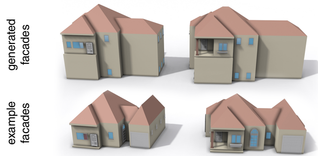
Figure 5.13: Results of applying an operations tree learned from unrepresentative examples. The operations tree for a family house was learned on single-floor buildings (bottom row). When applied to two-floor buildings, there is ambiguity that results in unexpected element placements (top row). Providing additional examples on two-floor buildings would help resolve the ambiguity.
