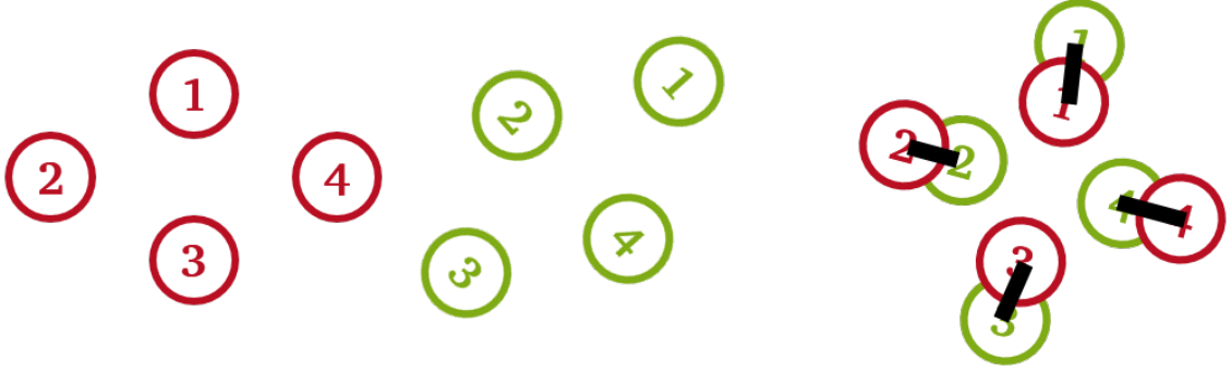
Figure 3.21: Rotating one of the two point clouds (green) reduces the average distance between pairs.
