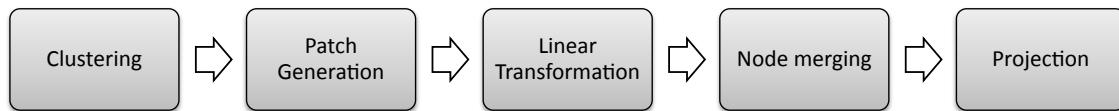
Figure 3.32: The original graph is first partitioned into clusters which are then used to create overlapping patches. For each pair of overlapping patches a linear transformation is computed that brings shared nodes together. They are then merged before they are projected into screen space.
