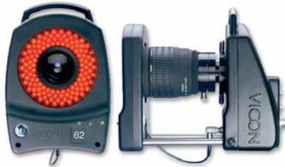
Figure 26: A Vicon MX camera, with infrared emitters and filter
