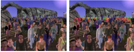
Figure 6: (left) Virtual humans navigating in a complex environment. (right) Similar image with apparent levels of detail; in red: the rigid meshes, in green: the impostors.
