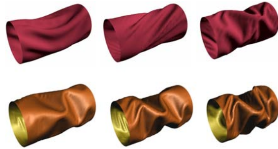
Figure 15: Top: Different types of folds on a garment's sleeve generated using a typical textile material. Bottom: Sequence taken from an animation of axial compression of a cylinder with a metal-like material.
