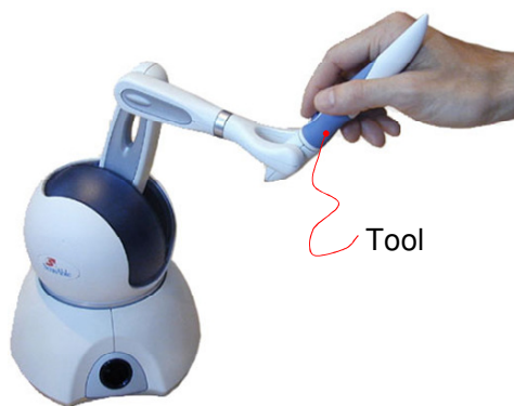
Figure 21: Picture of a force feedback device for the simulation of indirect interactions.
