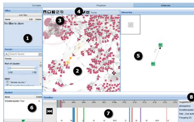
Figure 3.21.: The semantics visualization approach by VOIGT et al. with the different visualizations and interaction techniques: (1) data filtering, (2) the relational view on the uploaded data, (3) the mini map for overviewing the zooming area, (4) different relational graph-layouts and key-concepts selection, (5) hierarchical view, (6) the basket to remember instances of interest, and (7) a time-line for user interactions ([VPM13])
