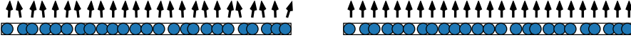
Fig. 3. Normal computations of an irregularly sampled boundary. Top: SPH normal computation using Eq. (33). Bottom: Corrected normal computation using MLS.
