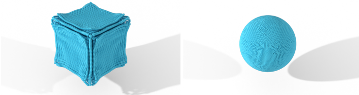
Fig. 8. Droplet formation in zero gravity using the surface tension model of He et al. without atmospheric pressure. The uncorrected version on the left suffers from artifacts through the double interpolation and the erroneous normal estimation while the corrected version on the right successfully forms a sphere.
