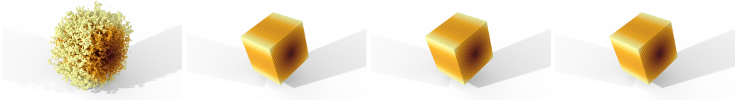
Fig. 6. A particle sampled cube placed in an external, rotational velocity field. Only the viscous force model by Takahashi et al. [2015] affects the particle’s motion. From left to right: uncorrected, KGC, MLS, RKPM. Only the uncorrected version introduces ghost forces which disintegrate the cube. The particles are shaded according to the velocity magnitude, with increasing values from dark to light.
