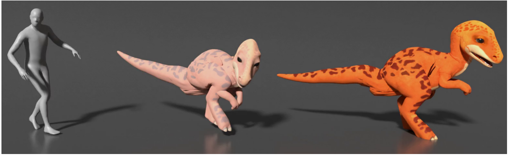
Fig. 4. Training data is generated through kinematic retargeting. The left character is the human mocap data. The middle character shows a rough kinematic retargeting by matching selected joint angles. This pose has many artifacts, such as feet sliding due to different leg lengths, self-collisions, floor collisions, and no motion of the tail and ears. The right character is the closest simulated pose that also respects all physical constraints. Notice how the head does not perfectly follow the human, as it's heavier and takes more time to react, not having access to future information but only past and present.
