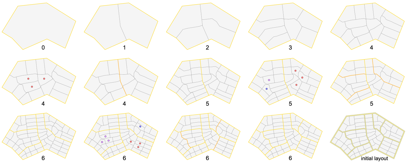
Figure 5: Our hierarchical approach that co-generates parcels and streets. The number below each subfigure is the corresponding hierarchical level (e.g., the input polygon is at level 0). In levels 1, 2, and 3, all the new parcels are reachable by the existing street network (colored in yellow). Hence, there is no need to generate new streets. In levels 4, 5, and 6, we identify and group unreachable parcels with the existing street network, where parcels in the same group are highlighted with dots of the same color. Then, we generate new streets (colored in orange) to create a street access for each unreachable parcel.
