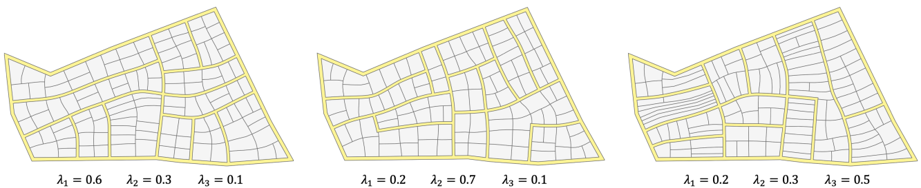
Figure 13: Our framework allows controlling parcel shapes by adjusting the three weights in the streamline quality metric (see Equation 2); e.g., the middle layout has more regular parcels, and the right layout has some elongated parcels for sharing the same street access.
