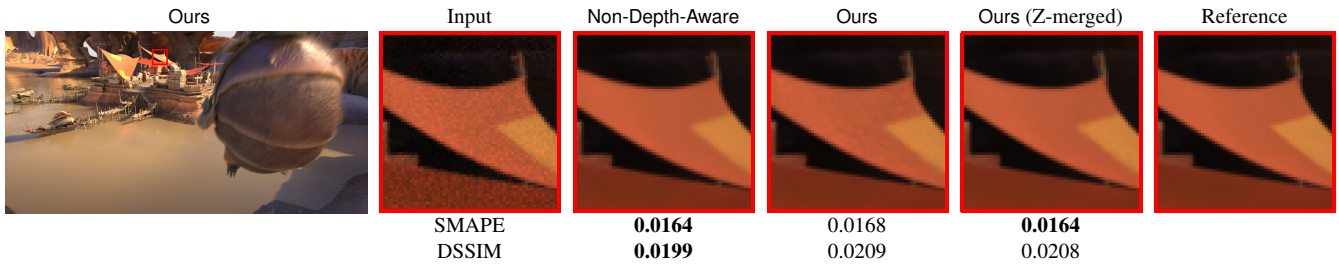
Figure 11: Failure case of depth-aware neighborhood when multiple bins are created for a single slanted surface. By merging bins based on depth more aggressively, the artifact can be mitigated, suggesting the potential benefit of more advanced binning and indexing methods. © Disney
