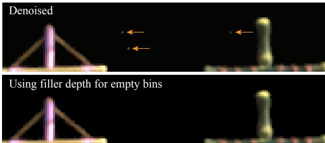
Figure 14: Depth denoising artifacts (top) and result after using filler depth for empty bins (bottom). The results are shown for a 32spp input image with the background removed. © Disney
