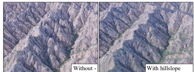
Figure 9: Close-up view on a ridge-line with hillslope disabled (left) and enabled (right). Hillslope controls the slopes and prevents the formation of sharp ridges and peaks.
