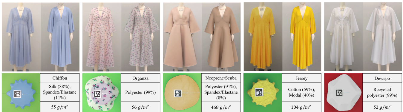
Figure 1: The line below shows Cusick drape test results and tag info for five actual fabrics. The tag information includes fabric type, fiber composition, and density. Using this data, we estimated optimal simulation parameters (stretching and bending) to replicate each fabric's drape property in a cloth simulator. For verification, we made two dresses: one with real fabric and another with the estimated parameters in a virtual environment. In the upper line, each pair consists of a real-fabric dress (left) and a virtually simulated dress (right).
