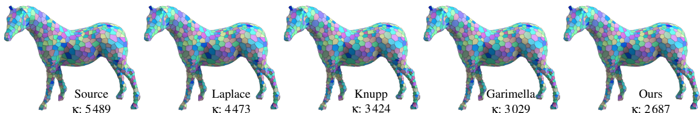
Figure 13: 2D manifold smoothing results on a mixed polygon mesh using Laplace smoothing, Knupp's [Knu00], Garimella's [GS04], and our method; all using surface Quadrics, respectively. GETMe is not included as the official implementation only supports 2D input.
