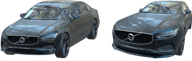
Figure 3: Vertigo effect. Left: The camera has a narrow FOV and is located far away from the car. Right: The camera has a wide FOV and is located close to the car. Notice how the car has the same projected size in both cases. We model the corresponding ambiguities in the distribution of cameras to yield distortion-free 3D shapes that look plausible from any viewpoint.
