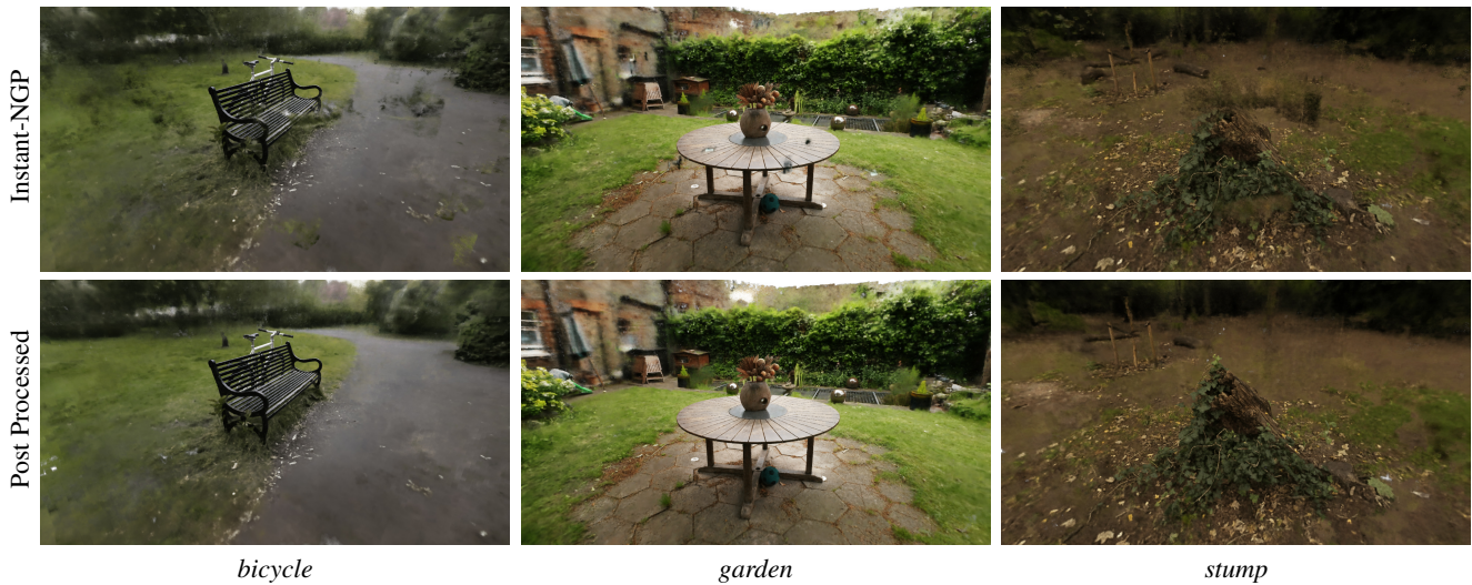
Figure 4: MIP-NeRF 360 scenes ‘bicycle’, ‘garden’ and ‘stump’ shown before and after our post processing approach [BMV*22]. Floating artifacts can be observed occluding the street (left), the table (middle) and the stump (right). Our clustering approach successfully removes these artifacts without impacting the integrity of the remainder of the scenes, improving the resulting image quality.
