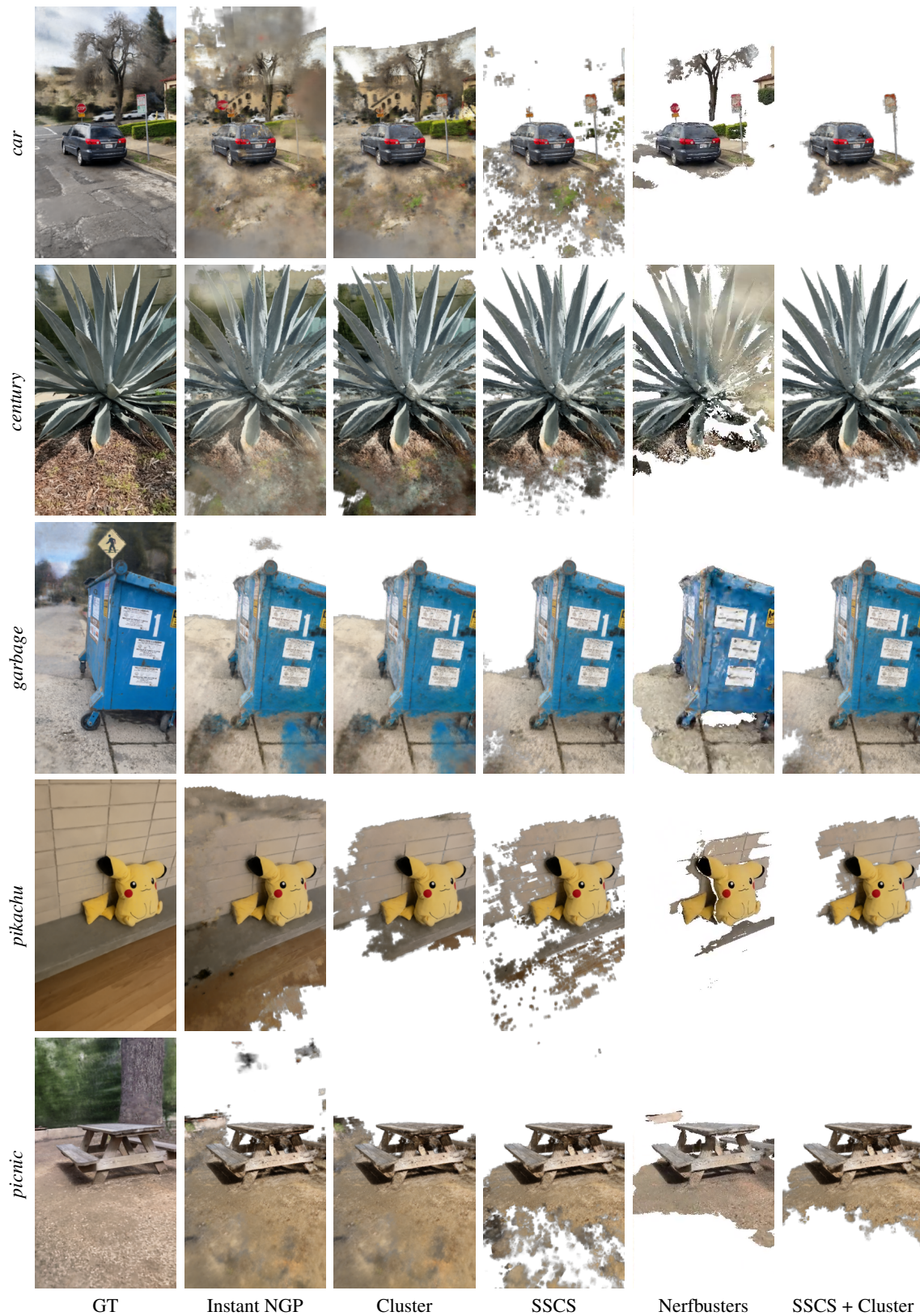
Figure 5: Evaluation views of the Nerfbusters scenes ‘car’, ‘century’, ‘garbage’, ‘pikachu’ and ‘picnic’. Renders of the Pseudo-GT Instant-NGP model, the unprocessed Instant-NGP model using only training views, renders using post-processed grids with only Occupancy Clustering and SSCS, the Nerfbusters renders by Warburg et al. [WWT*23] and our combined strategy are shown side-by-side.
