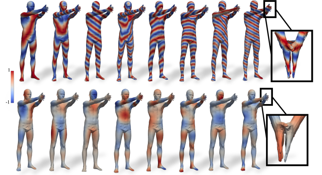
Figure 2: Comparison of Random Fourier Features (RFF) (top) and LBO Eigenvectors (bottom) for a FAUST subject. The intrinsic nature of the LBO eigenvectors, which account for mesh connectivity, makes them well-suited for representing indicator functions capable of isolating semantically meaningful body parts, such as a single hand, even when both hands are close in the Euclidean domain.
