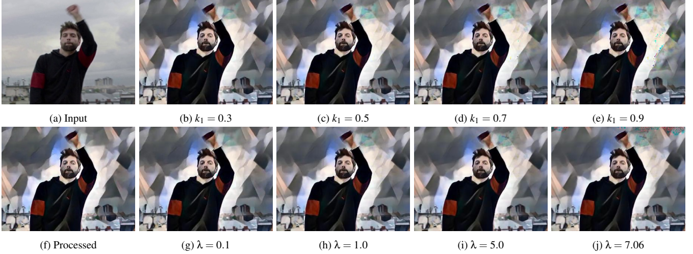
Figure 3: The level of consistency in the final output can be controlled via parameters k_1 and \lambda . Here we show how the final result varies by increasing these, for lower values the consistency is negligible and the results (Fig. 3b and Fig. 3g) visually look similar to the per-frame processed output (Fig. 3b). For higher values, we start observing artifacts due to ghosting and/or optimization (Fig. 3e and Fig. 3j).
