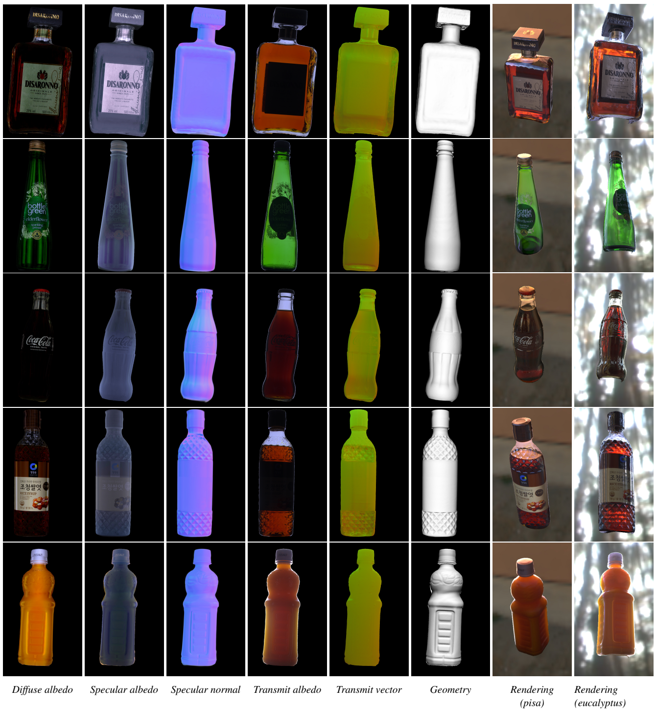
Figure 8: Results of acquired shape and appearance maps of reflective and translucent objects and 3D rendering in novel lighting environments.
