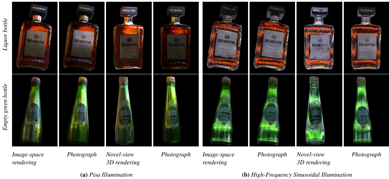
Figure 10: Rendering validation with actual photographs. The image-space renderings are created by directly using the captured reflectance images (as shown in Figure 5). For image-space rendering, we validate how our captured reflectance maps allow us to create a realistic rendering for that specific view. For novel-view 3D rendering, we test how well the learned 3D reflectance maps interpolate to an unseen novel viewpoint.
