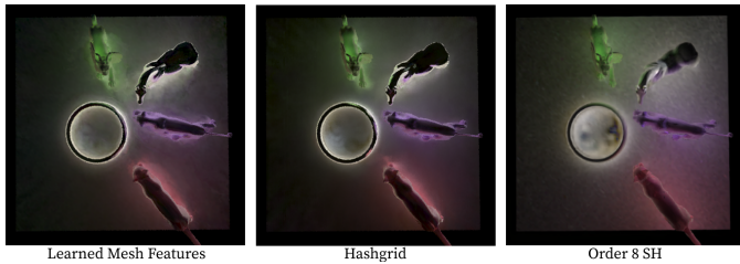
Figure 7: Ablation study on storing the learned feature vectors on mesh vertices (learned and SH) vs a hashgrid. Spherical harmonics with a maximum degree of 8 stored on mesh vertices [SKS02] are unable to properly represent caustics and the sharp reflections on the horse as expected, and also show some ringing and other artifacts. The learned mesh vertex features, while much better than SH, still cannot properly represent caustics, show a lot more noise in the reflections around the griffin and horse, and require a well-subdivided mesh. The use of the hashgrid solves these issues while being invariant to scaling of the scene.
